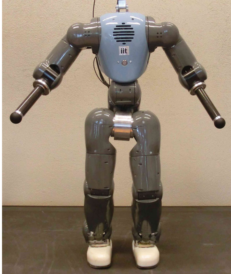
Fig. 1. Compliant HuMANoid Platform—COMAN, developed by IIT, and used in the experiments to demonstrate the possibility of using modified task space control for motion imitation.
