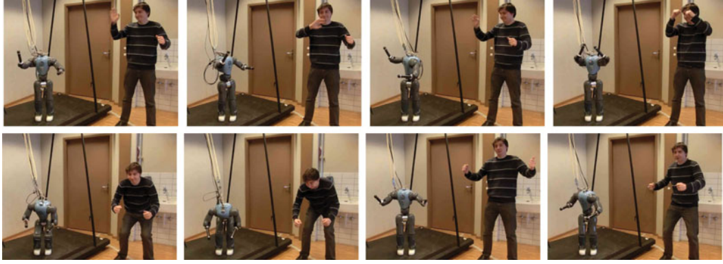
Fig. 7. Sequence of images showing real-time motion imitation with the robot while maintaining stability. The demonstrator performed random waving, squatting, and bending motions, but maintained the double feet support at all times.
