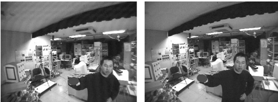
Fig. 2. The detected right human hand overlaid by the estimated blob as seen by left and right eye.
