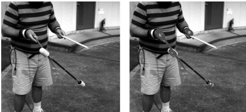
Fig. 1. Observing the devil sticking: (left) input; (right) result. Five blobs were tracked simultaneously.
