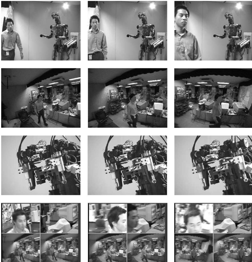
Fig. 5. Smooth pursuit with DB's left eye. First row shows the action taken by the external camera, second row shows successful face tracking while the camera is moving (the face is overlaid with the detected blob), third row shows how DB's left eye is moving, and fourth row shows the view from all four cameras demonstrating that the person's head stays within the viewfield of the left narrow-view camera.
