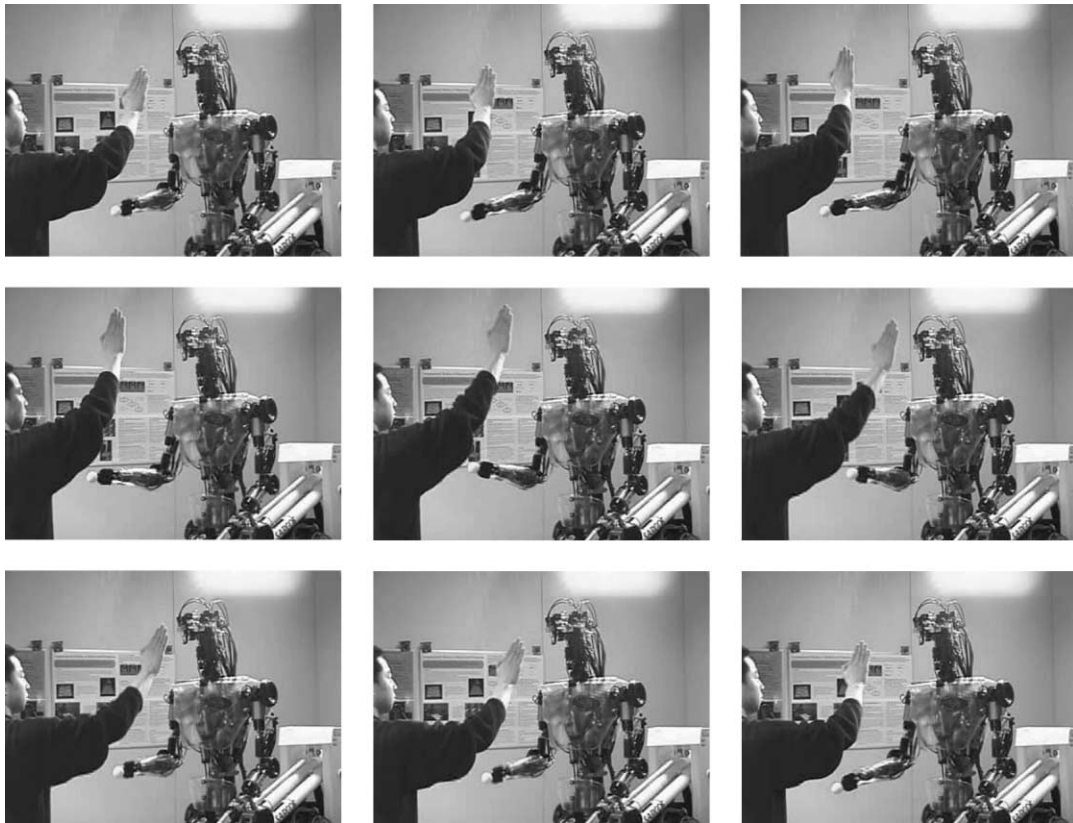
Fig. 3. DB mimicking hand motion. Every tenth frame from a video is shown.
