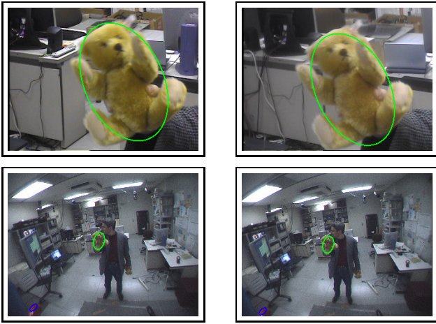
Fig. 2. Tracking in peripheral and foveal images. The green ellipses show the detected locations and shapes.
