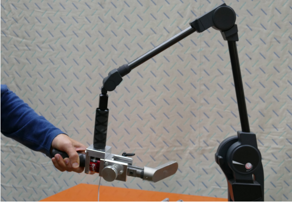
Fig. 1. Learning by demonstration setup for polishing/grinding.
