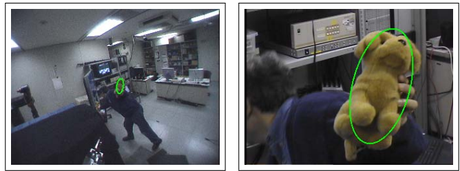
Fig. 5. Maintaining the object view in foveal image based on information from the peripheral view
