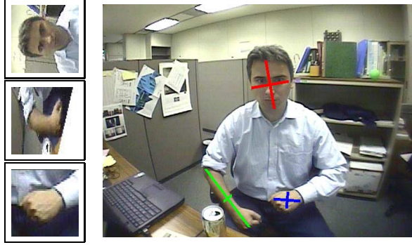
Figure 1. Warping three regions around the tracked body parts. The original image overlaid with the estimated blobs (displayed as crosses) is also shown.
